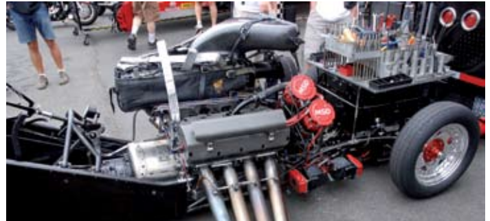
From the rear motor plate back, chassis specifications are very rigid. There are two options for main rails from the motor plate back: Double rail or triple rail. From the plate forward, the chassis builder can become slightly creative. Distance between the main rails has an effect upon performance
