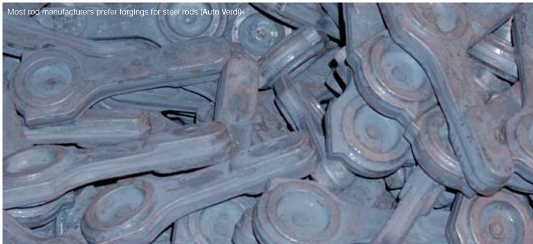
Most rod manufacturers prefer forgings for steel rods (Auto Verdi)
